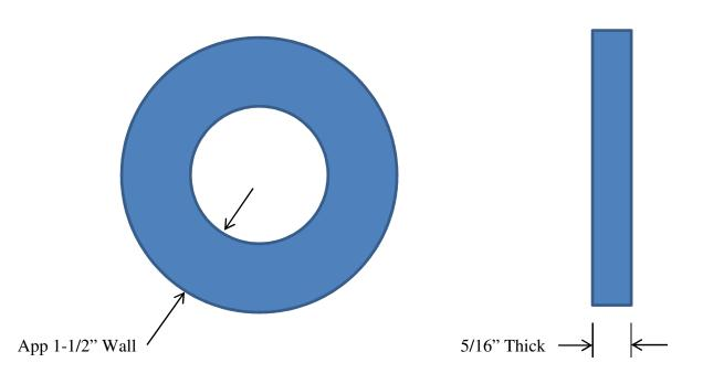
At the time of an order, the customer will need to furnish the nominal pipe inside diameter and percentage interference. For example a 10 Standard Wall Pipe = 10.020" ID, with a 2% interference, yields a desired sizing ring diameter of 10.220". Or, if the actual internal diameter of the ring is known, the finished part can be cut to the specified size.
